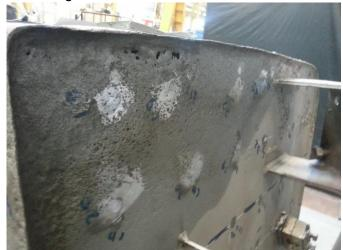
Bottom of corroded diesel tank featuring pitting and holes
