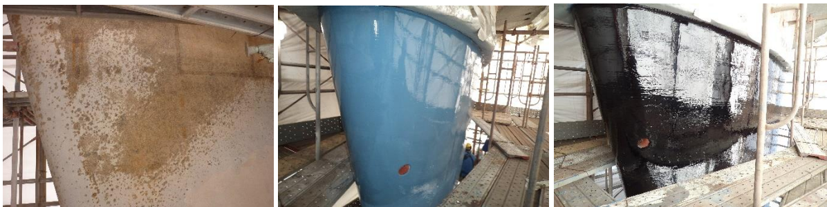
Belzona cavitation protection system application to a Naval vessel in Japan
