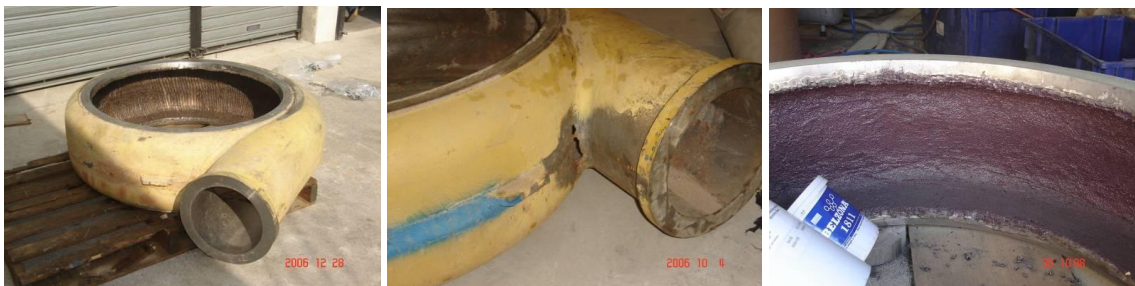
Pump repair and abrasion protection at a Guatemalan gold mine
