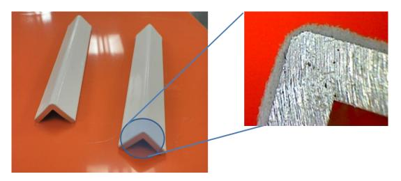
Figure 5: Excellent edge retention - NACE TM0304 specified 90° angle aluminium specimen with ridge radius curvature of 0.7mm. The peak to flat coating thickness ratio of 0.5 is achieved
