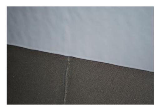
Figure 4: Single coat application of Belzona 1331 achieves full coverage of a 1.5mm high weld bead. The masking tape was removed to reveal the weld bead.
