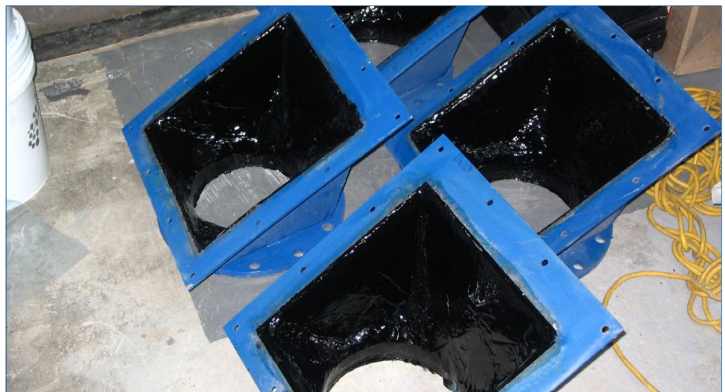
Hoppers lined with Belzona 2111
