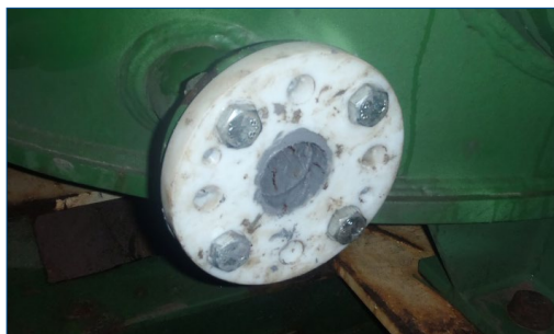
Former in place with Belzona material
