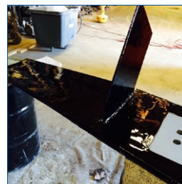
Protection of agitator blade
