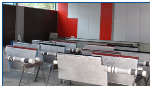
Long-term erosion-corrosion protection of the leading edge
