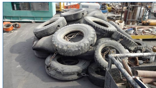
Initial inspection of deflated fender
