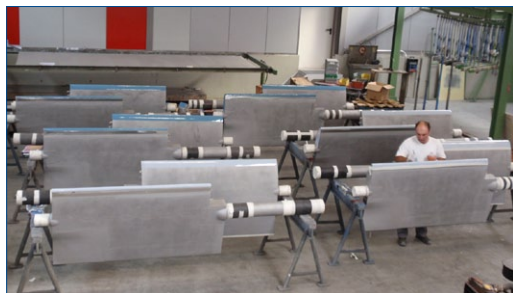
Wicket gates after blasting and initial application
