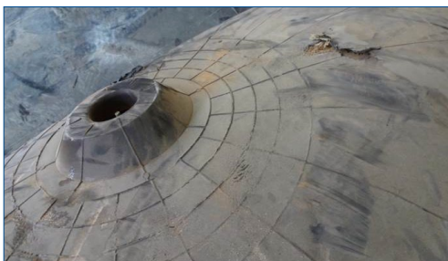
Torn rubber fender
