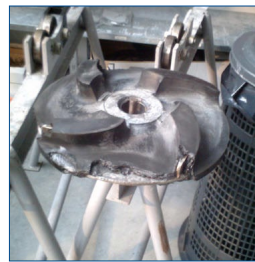
Rebuilt rubber impeller
