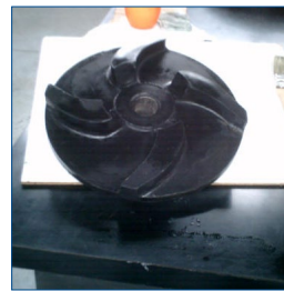
Rebuilt rubber impeller
