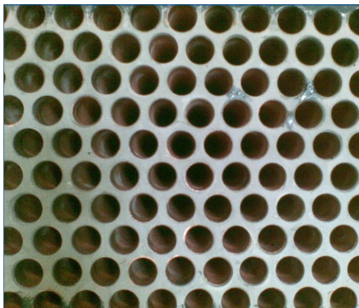
Close-up of the coated tube sheet
