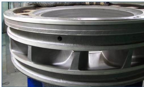
Blasted runner prior to the application
