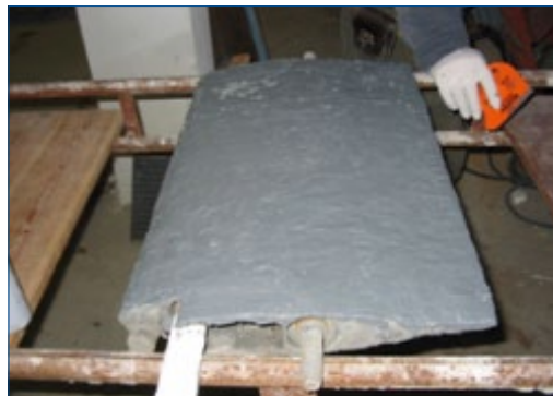
Blade after rebuilding with Belzona 1111 (Super Metal)
