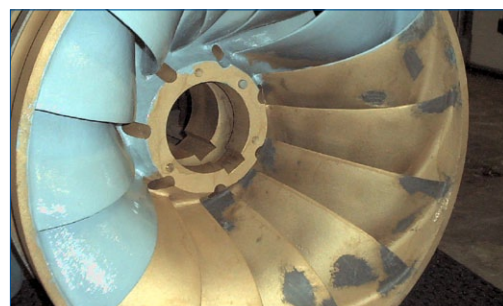
Turbine following rebuild using a paste grade material to in-fill areas of erosion damage
