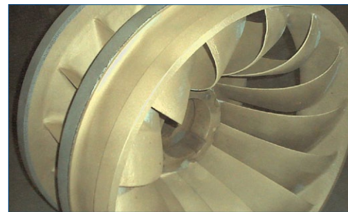
Francis turbine following preparation by grit blasting
