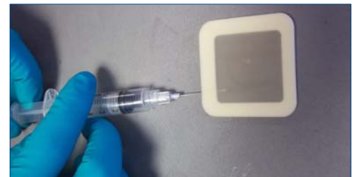
Thorough inspection for salt contamination (including chloride concentration measurement) ensures optimum surface preparation
