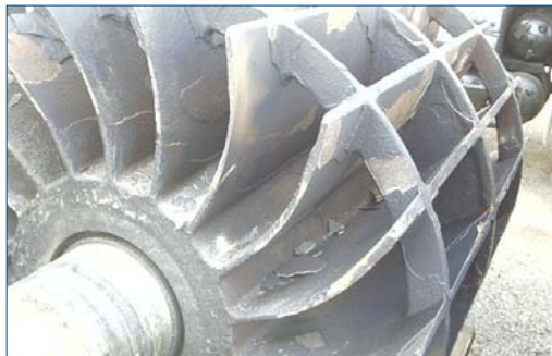
Rotor before application of the Belzona 1311 (Ceramic R-Metal) and Belzona 1321 (Ceramic S-Metal) system
