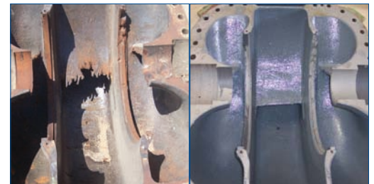
Typical effects of erosion-corrosion on a centrifugal pump cutwater After rebuilding and coating with Belzona
