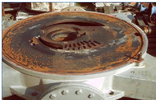
Port plate before application with Belzona 1111 (Super Metal)
