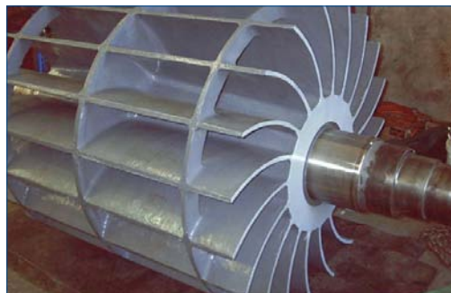
After application of the Belzona 1311 (Ceramic R-Metal) and Belzona 1321 (Ceramic S-Metal) system
